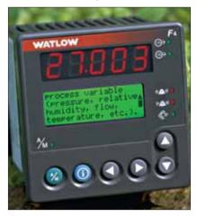
Available in ½2, ½6, ½ and ½ DIN sizes, agency approved Watlow single-loop, auto-tuning temperature controllers automatically set PID control parameters for optimum system performance. Manual settings also permit on-off, P, PI or PID control modes. All Watlow auto-tuning controllers are designed and manufactured to withstand harsh industrial environments and come with a three-year warranty for Control Confidence®.
