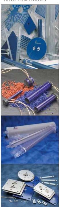
Watlow layers thick film resistor and dielectric materials on quartz, stainless steel and ceramic substrates to produce high performance industrial heaters. The thick film heaters provide very fast temperature response and fine thermal uniformity on a low-profile heater. Thick film heaters are ideal for applications where space is limited, where conventional heaters can't be used, when heat output needs vary across the surface, or in ultra-clean or aggressive chemical applications.
