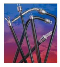
The multicell heater from Watlow offers independent zone control for precise temperature uniformity, loose fit design for easy insertion in and removal from the equipment and extreme process temperature capability. The heaters are available with up to eight independently controllable zones and one to three internal thermowells for removable sensors. Custom assemblies are available.
